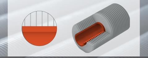
**Type I-Fin** is a type of tube where the fin is coiled around the core tube with to ensure the fin-to-tube contact. The ends of the fin are tackwelded on the tube. Due to its smooth fin surface the air sided pressure drop is very low even at high air velocities.
