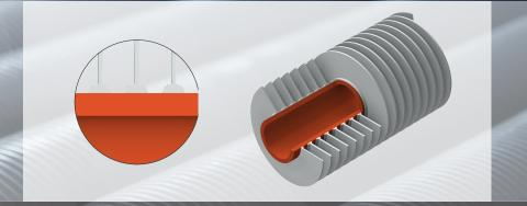
**Type S-Fin** is a type of fin tube where the fin is welded circumferentially on a core tube by high-frequency welding.
