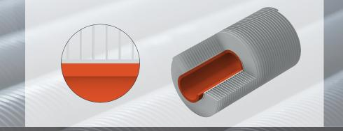
**Type E-Fin** is a type of fin tube where the fin is rolled from a hollow blank aluminium tube slid over the core tube by a process using pressure to create a rolled "pressure bond" between the core tube and fins.
