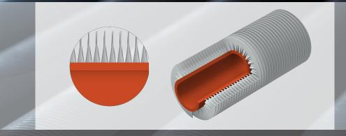
**Type W-Fin** is a type of fin tube with a fin which has a corrugated shape at the foot of the fin. It is coiled around the core tube with a certain pre-tension to ensure an ideal fin-to-tube contact. The ends of the fin are tackwelded on the tube.
