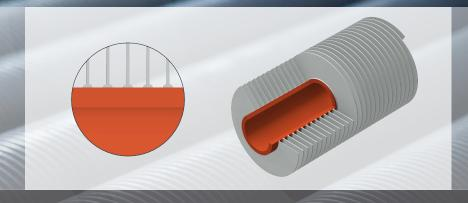
**Type LF-Fin** is a type of fin tube which consists of a circumferential stainless steel or aluminium fin which is welded spirally on a stainless steel core tube by means of a laser.
